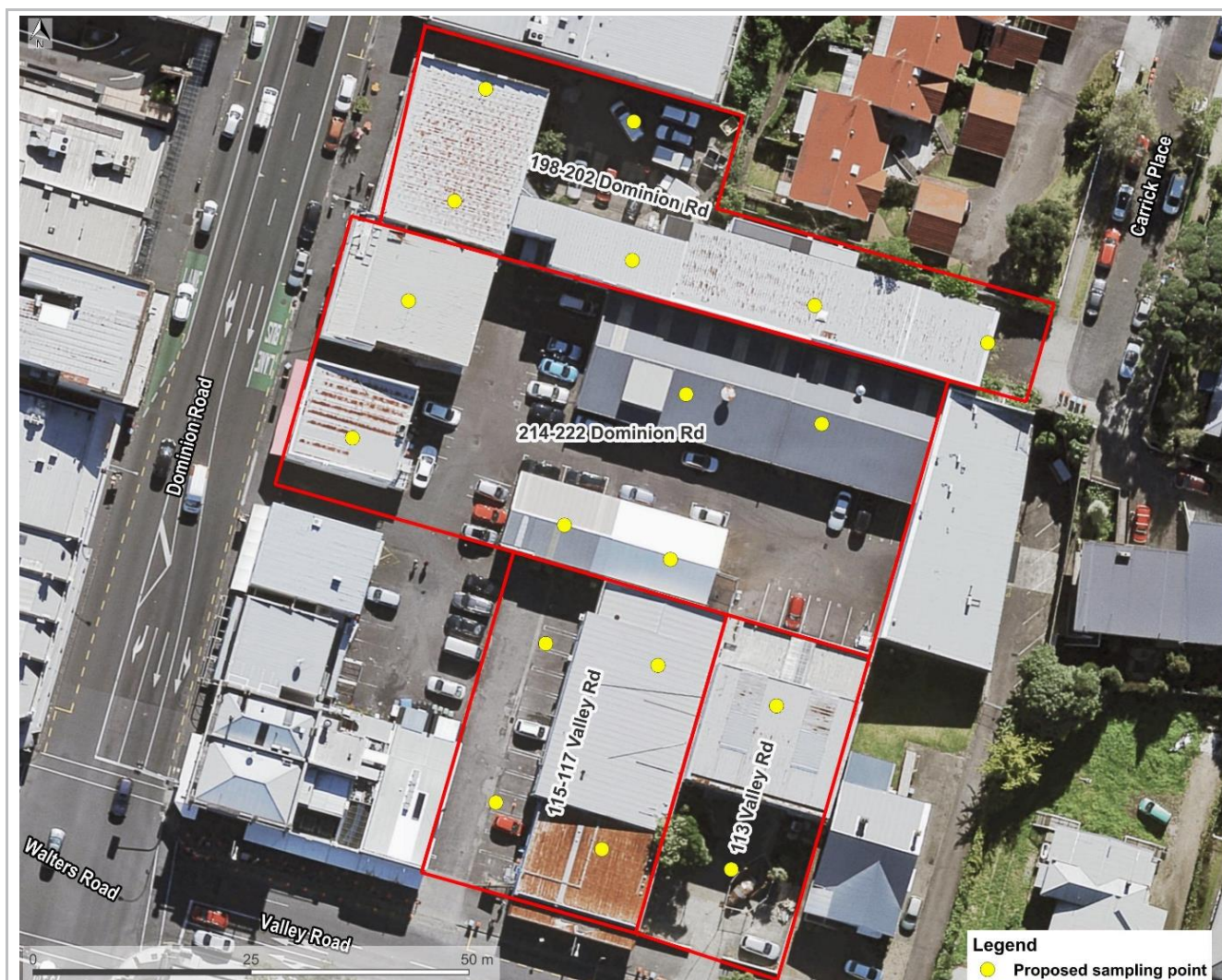
Figure A1: Post-demolition investigation plan to be implemented by the SQEP .
